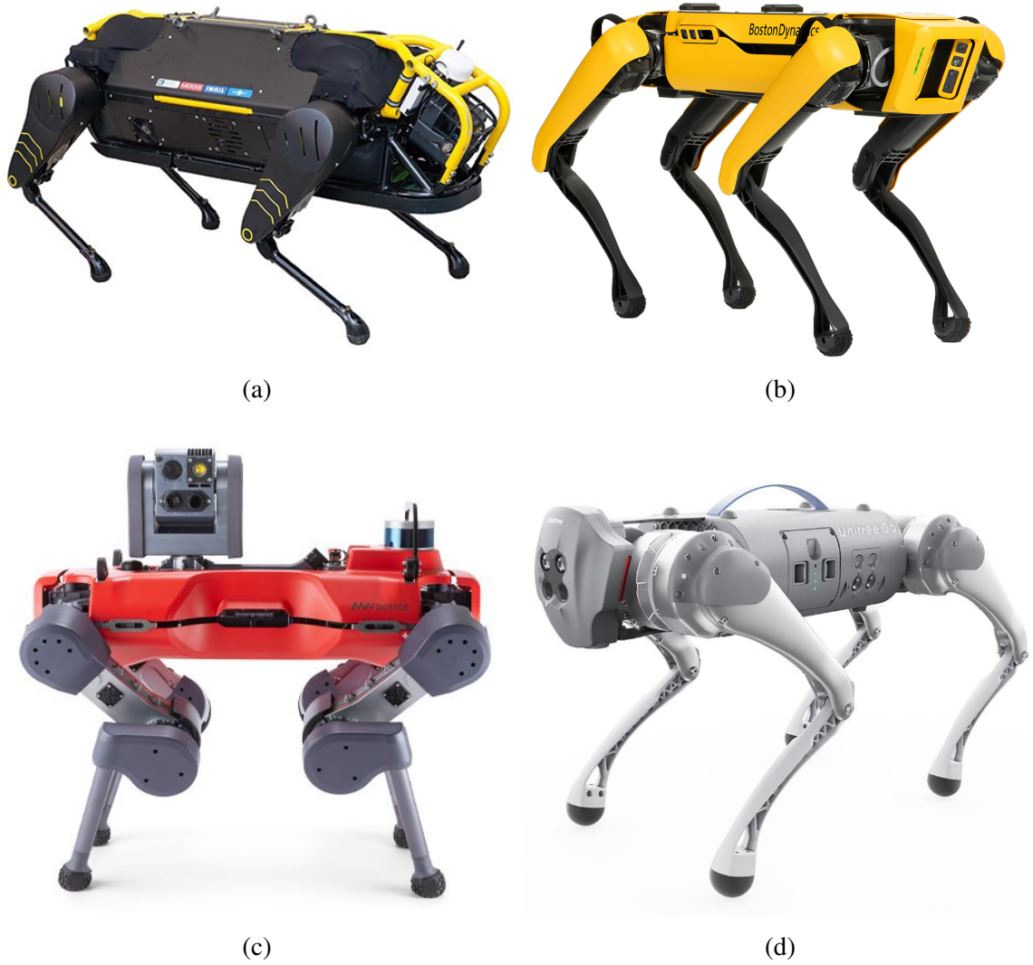
Figure 2.1 Quadruped robots: (a) Istituto Italiano di Tecnologia (IIT) HyQReal, (b) Boston Dynamics Spot, (c) ANYbotics ANYmal, and (d) Unitree Go1.
