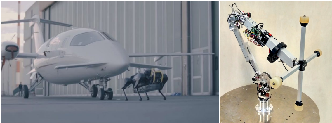
Figure 4.3: Left: Hyq2Max [98] demonstrates the power of hydraulic actuators by pulling a three-ton plane; right: a high-performance balancing robot equipped with small and fast brushed DC motors (see Section 5.5).
