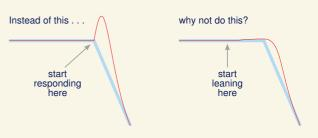
This behaviour can be implemented by changing the command input to the controller.
