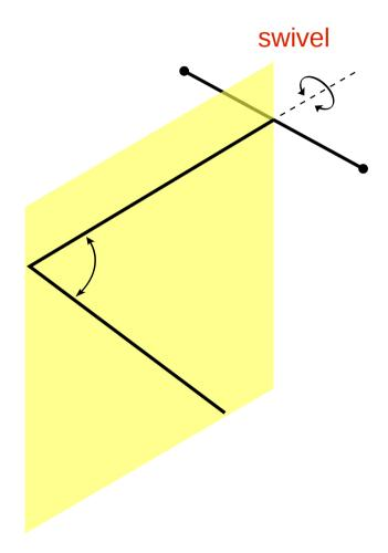
Keeping the balance plane vertical is accomplished by *rotating the crossbar*. In addition to keeping the balance plane vertical, this '*swivel*' controller can also
