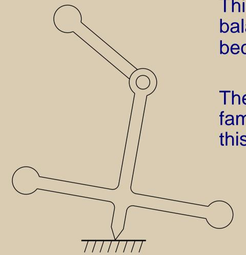
This mechanism cannot balance in any configuration because  $G_v = 0$  everywhere.
